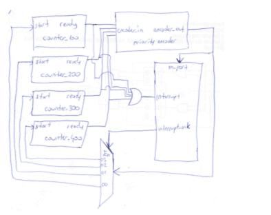
When interrupt is asserted, s1 register will give the counter number of interrupt in interrupt subroutine. When more than one interrupt is received, s1 register will give output of priority encoders. For priority\_encoder.v and conter.v please contact eabtioglu@gmail.com
