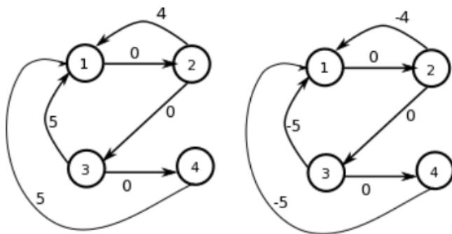
$G_d$  has  $d$  nodes where each nodes corresponds to one of the delay in  $G$ ,  $w_{i,j}$  is the longest path length among all the path in  $G$  (do not pass through any delay!)
