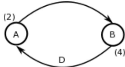
Node  $A$  represents addition and Node  $B$  represents multiplication. And edges represent data path, note that edge  $B \rightarrow A$  has one delay.
