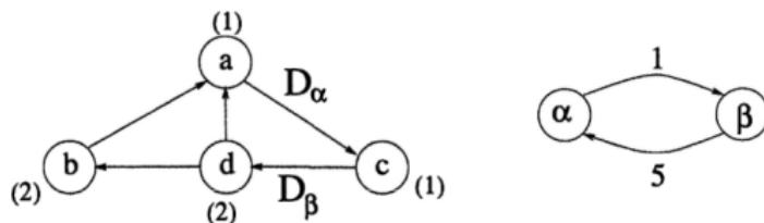
Two cycles contain the delay  $D_\alpha$  and  $D_\beta$  in  $G$  and their comp. time 6 and 4 u.t.
