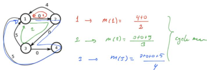
The maximum cycle mean of  $G_d$  is the maximum cycle bound of all cycles in  $G$  which is the iteration bound of  $G$ .
