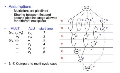
Minimize latency under resource constraint (a1=3 MULTs, a2=3 ALUs )
