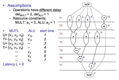
Minimize latency under resource constraint (with  $d_1 = 2$ ,  $d_2 = 1$ )
