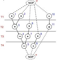
Minimize latency under resource constraint (with d = 1)
