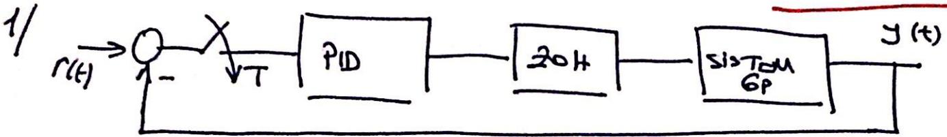
$$G_p = \frac{1}{s(s+1)}, \quad PID = K_p + \frac{K_I}{1-z^{-1}} + K_D(1-z^{-1})$$
