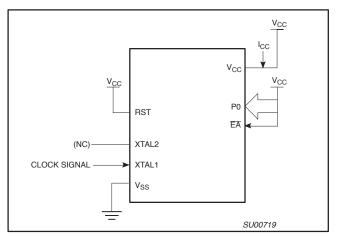
Figure 22. I<sub>CC</sub> Test Condition, Active Mode All other pins are disconnected
