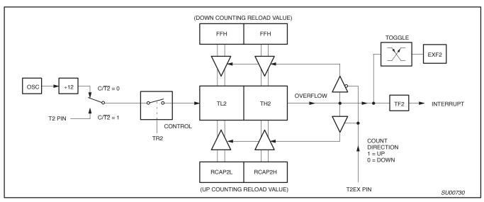
Figure 5. Timer 2 Auto Reload Mode (DCEN = 1)
