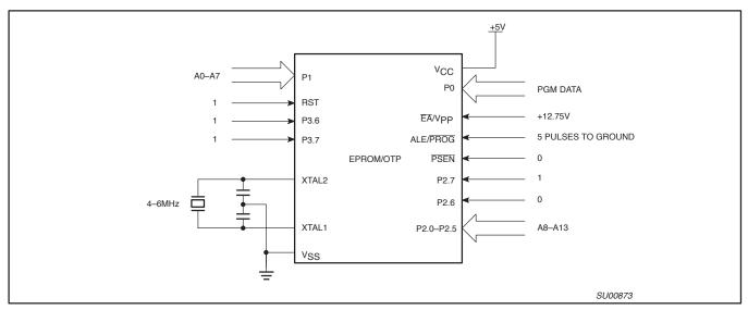
Figure 26. Programming Configuration
