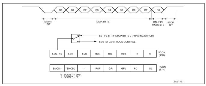
Figure 8. UART Framing Error Detection
