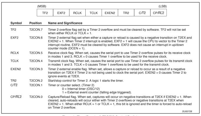
Figure 1. Timer/Counter 2 (T2CON) Control Register
