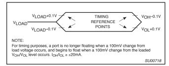
Figure 20. Float Waveform
