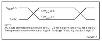
Figure 19. AC Testing Input/Output
