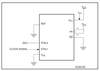
Figure 23. I<sub>CC</sub> Test Condition, Idle Mode All other pins are disconnected
