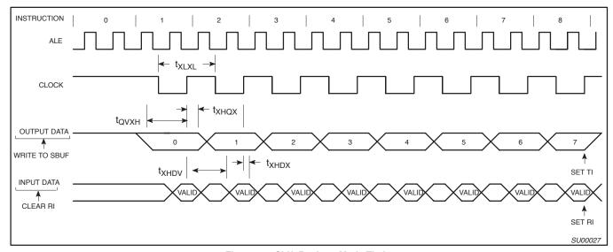
Figure 17. Shift Register Mode Timing
