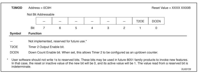
Figure 3. Timer 2 Mode (T2MOD) Control Register
