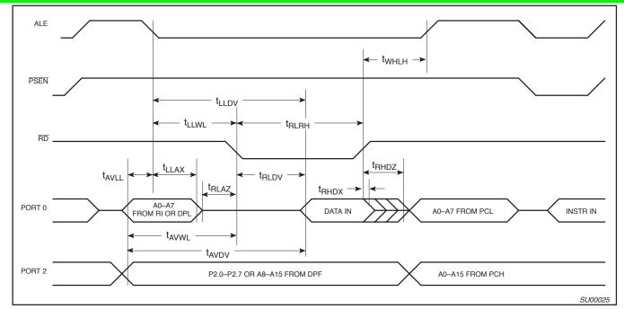
Figure 15. External Data Memory Read Cycle
