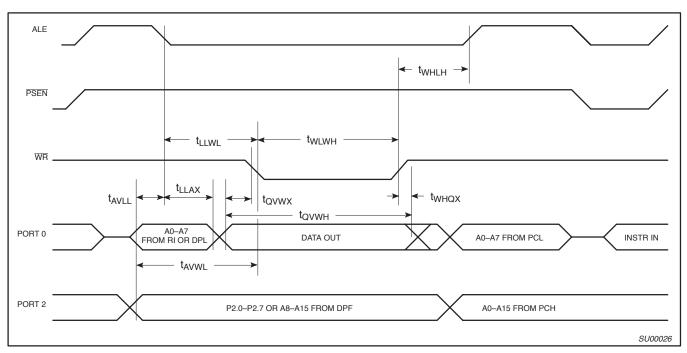
Figure 16. External Data Memory Write Cycle
