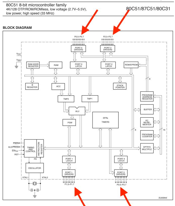
80C51 8-bit microcontroller family 4K/128 OTP/ROM/ROMless, low voltage (2.7V–5.5V), low power, high speed (33 MHz)
