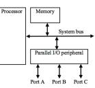
Adding parallel I/O to a busbased I/O processor
