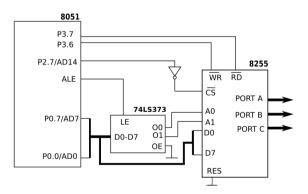
I/O port addresses assigned (memory mapped I/O) to ports A, B, C, and the control register:
