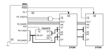
if  $\overline{EA} = 1$ , PC starts from 0000h(internal memory) then 0FFFh (external memory), if  $\overline{EA} = 0$ , PC start from external memory (0000h - ----h).  $\rightarrow$  8051, page 25 (external program memory read cycle)
