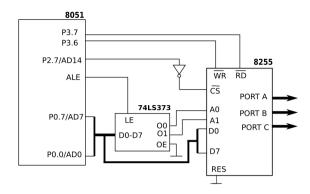
"All the ports of A, B and C are output ports " then the control word of the 8255 for the configurations ( 8255, page 3-100 ) is 1000000b=80h For P3.7 and P3.6 see • 80C51, page 6 and for 74LS373 (Latch) see • 74LS373. A program to send *FFh* to all ports:
