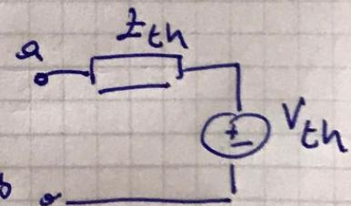
$$\textcircled{2} \quad Z_L = \overline{Z}_{th} = 4+4j = \frac{R_L + j\omega L_L}{4\omega} = \frac{4\Omega}{4H}$$
