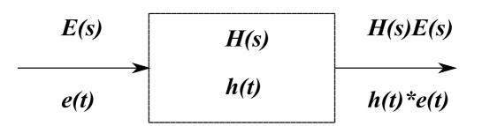
$\begin{array}{l} \mbox{impuls response} = h(t) = \mathcal{L}^{-1}\{H(s)\}\\ \mbox{step response} = h(t)u(t) = \mathcal{L}^{-1}\{H(s)\frac{1}{s}\}\\ \mbox{! zero-input response} = 0 \mbox{!}\\ \mbox{what happen if zero-input response is not zero (or system is not stable)?} \end{array}$
