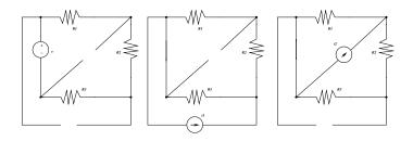
$y(0, i_1, 0)$  is equal to the response of y when all independent sources in the circuit except  $i_1$  are set to zero.
