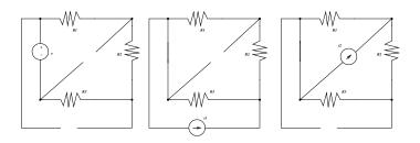
$y(0,0,i_2)$  is equal to the response of y when all independent sources in the circuit except  $i_2$  are set to zero.
