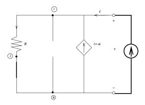
KCL for the node ①;  $-i + GV_{d1} - i_b = 0$ . Substitute  $i_b = \alpha G(V_{d1})$  into the KCL eqn.  $-i + GV_{d1} - \alpha GV_{d1} = 0$ . Then we obtain
