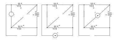
y(e, 0, 0) is equal to the response of y when all independent sources in the circuit except e are set to zero.
