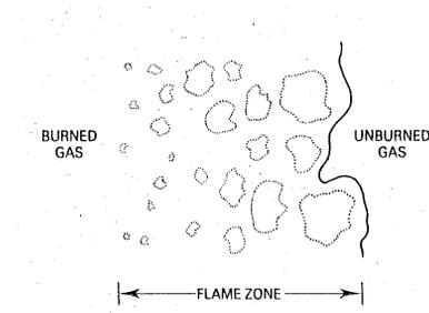
Turbulent flame speed is in the range of 50 – 60 m/s
