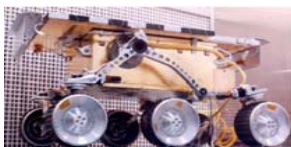
The 25-pound, six-wheeled robotic explorer
