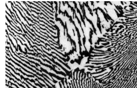
Micrograph of Pb-Sn eutectic microstructure
