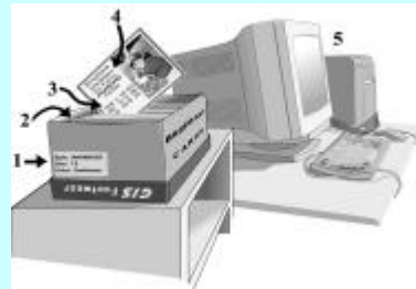
Figure 2.1 The Elements of a GIS. (1) The Database (shoobox); (2) The Records (Baseball Cards); (3) The Attributes (The categories on the cards, such as a batting average); (4) The geographic information (locations of the team's stadium in latitude and longitude); (5) A means to use the information (the computer).
