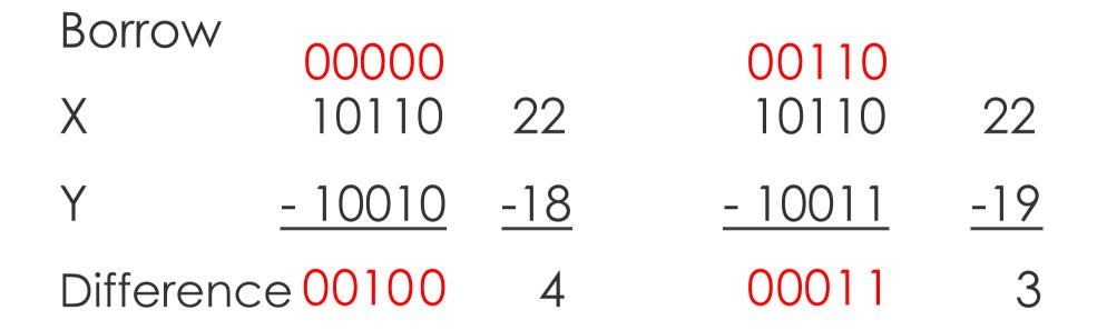
Note: The borrow input to the LSB is always '0'. If Y>X, then X and Y are exchanged and – sign is put in front of the result.
