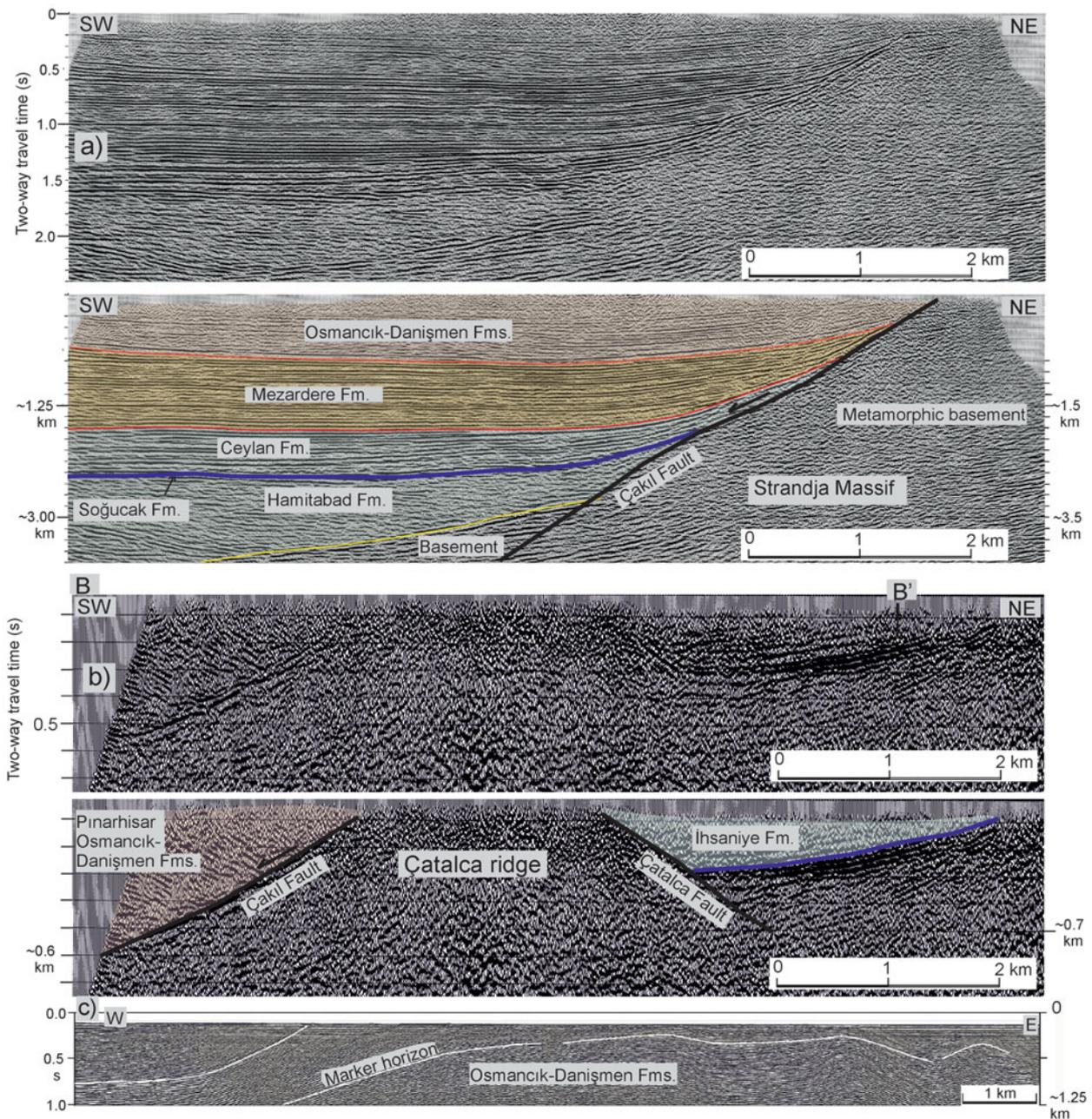
Figure 14. (Colour online) Time-migrated seismic reflection sections of lines (a) 88-34 and (b) MAD-90-311 perpendicular to the Çatalca ridge and (c) MCS02 in the Marmara Sea. For the location of the profile see Figures 2 and 13. Line MCS02 is modified from Ergintav *et al.* (2011).
