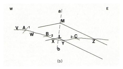
**Step 2:** To determine the trace of the hinge plane that passes through point L, bisect angle XLY. The hinge-plane trace is line *ab* (Fiğ. b).
