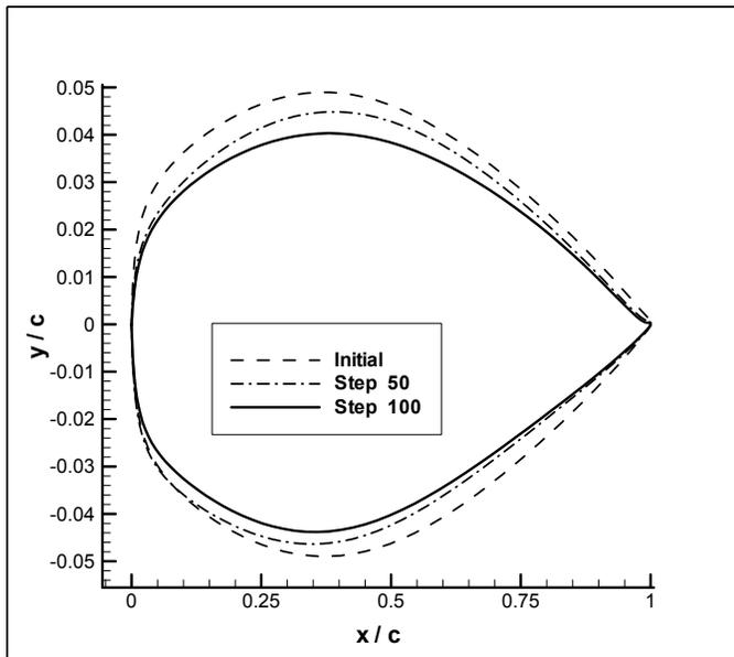
Figure 7: Wing sections of the first and the best members found at the steps 50 and 100
