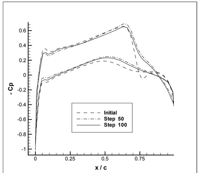
Figure 6: The Cp distributions of the root sections at different stages
