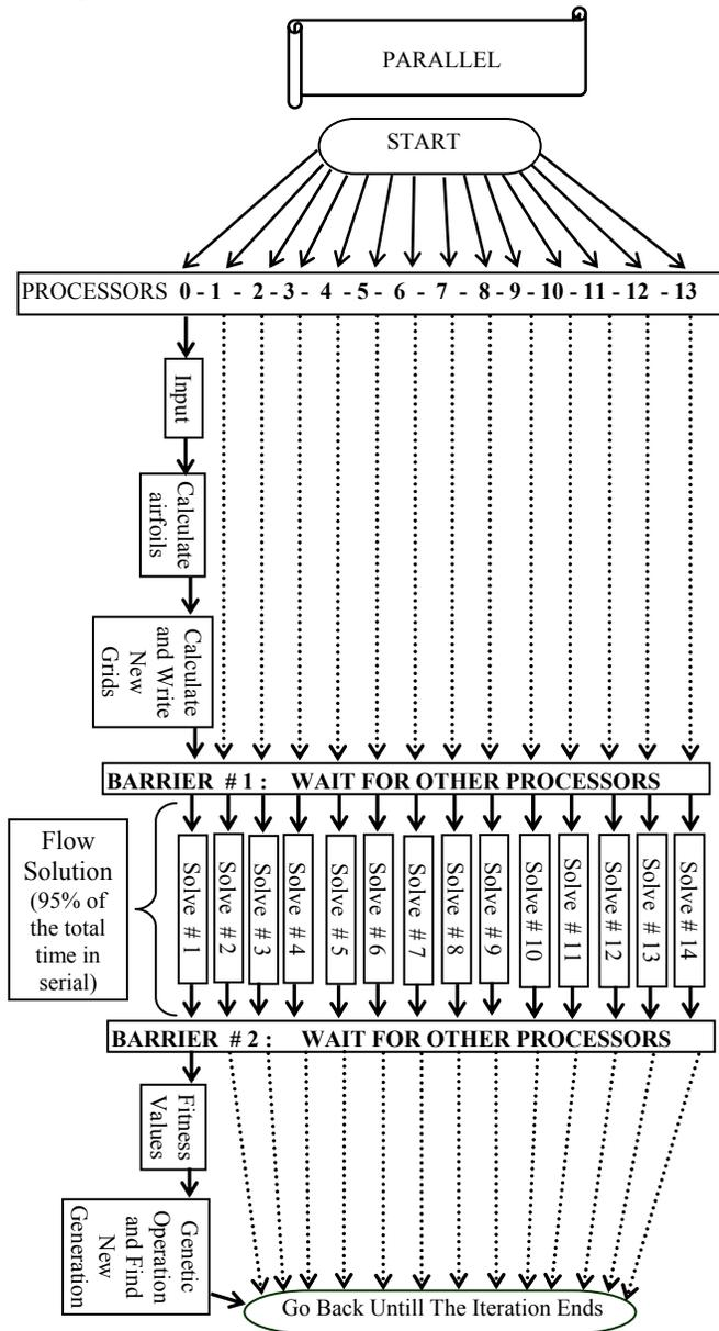
Figure 1: Main Structure of the Parallel Processing
