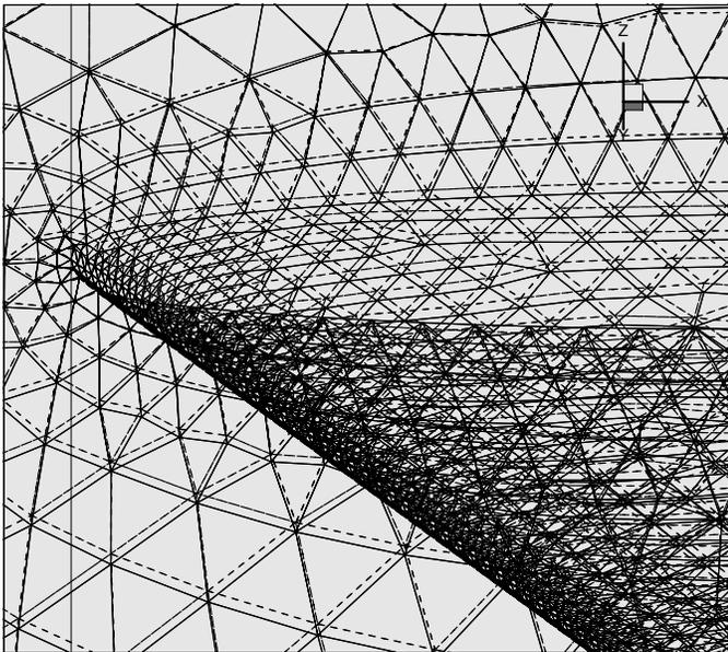
Figure 4 : The mesh structures of the first and the best wing found at the 100th population (initial: dashed line, 100<sup>th</sup> : solid line)
