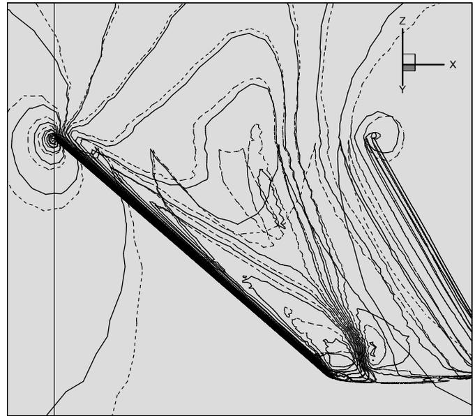
Figure 5 : The Cp distributions of the first and the best wing found at the 100<sup>th</sup> population (initial: dashed line, 100<sup>th</sup> : solid line)
