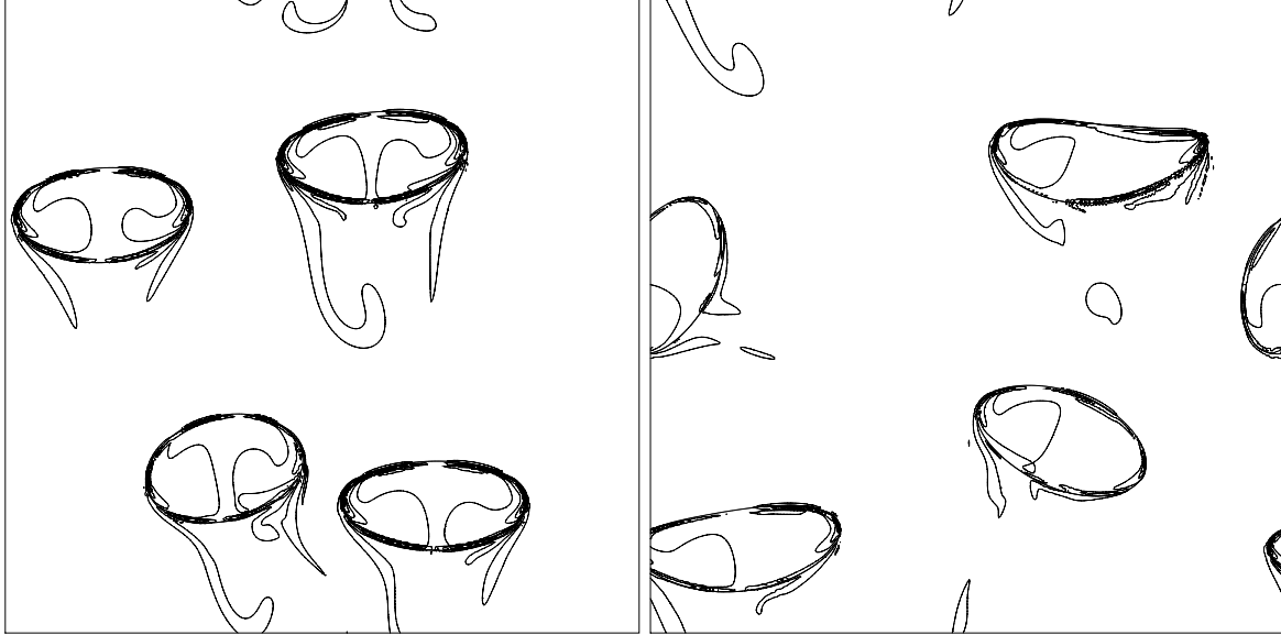
Figure 18: High Reynolds number bubbles at two times. The bubble surface and a few vorticity contours are plotted in each frame.
