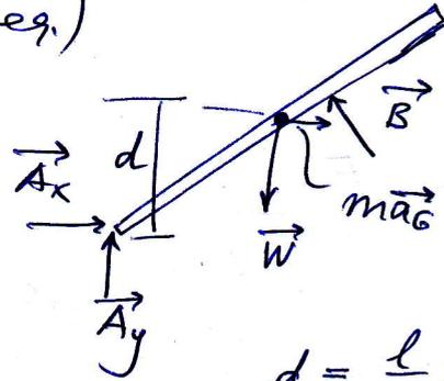
$$\begin{aligned}d &= \frac{l}{2} \sin \alpha \\ &= \frac{3.75}{2} \sin 26,4 \\ &= 0,833 \text{ m}\end{aligned}$$
