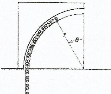
Calculate the velocity of the chain in decimals for  $\theta = 0$ ,  $\theta = 30^\circ$ ,  $\theta = 60^\circ$ , and  $\theta = 90^\circ$ .
