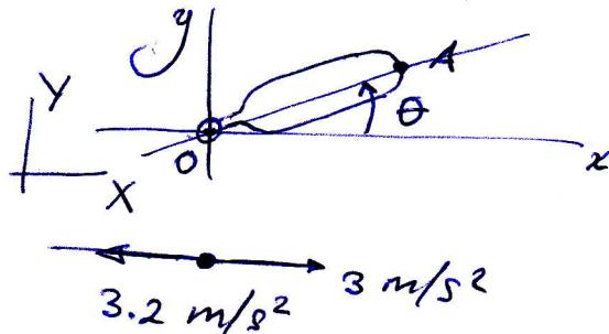
$$\vec{a}_A = \vec{a}_O + \vec{\alpha} \times \vec{r}_{OA} + \underbrace{\vec{\omega} \times (\vec{\omega} \times \vec{r}_{OA})}_{\text{normal acc.}}$$
