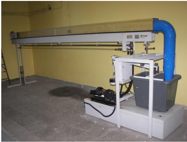
Photo 1. Laboratory free surface flow flume
