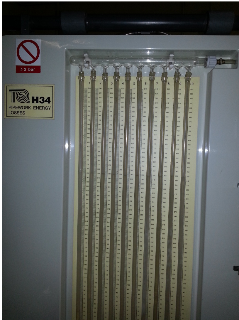
Figure 5: The piezometer tubes.
