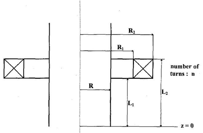
Fig. 2. Geometry of the problem with an  $n$ -turn coil.  $R = r_{N-2}$  is the radius of the workpiece.
