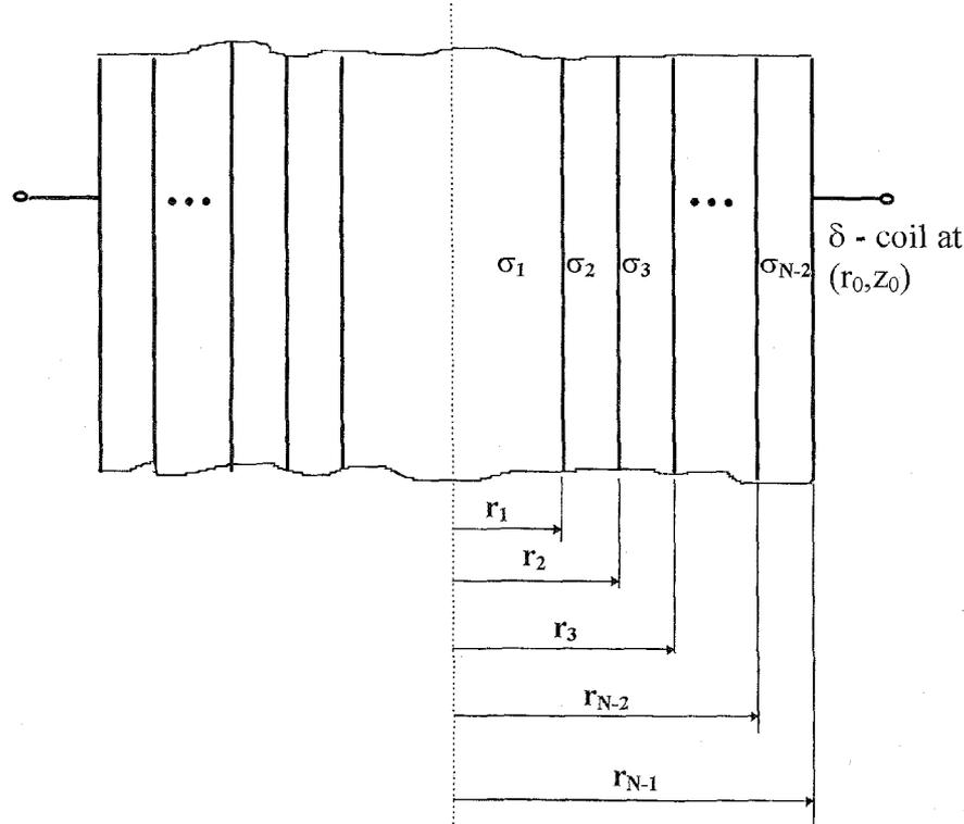
Fig. 1. Multilayered cylindrical workpiece surrounded by a single-turn coil.
