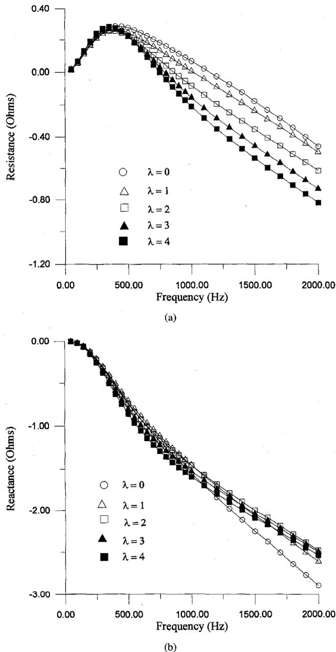
Fig. 4. (a) Real part of the impedance as a function of frequency for the profiles of Fig. 3. (b) Imaginary part of the impedance as a function of frequency for the profiles of Fig. 3.
