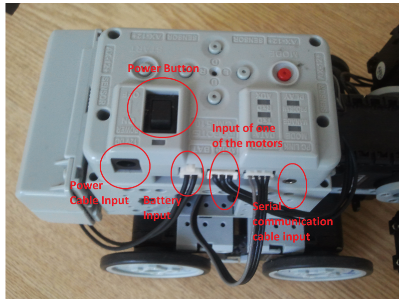
Figure 2.3: CM-510 controller of Bioloid and its connection inputs for the peripherals.
