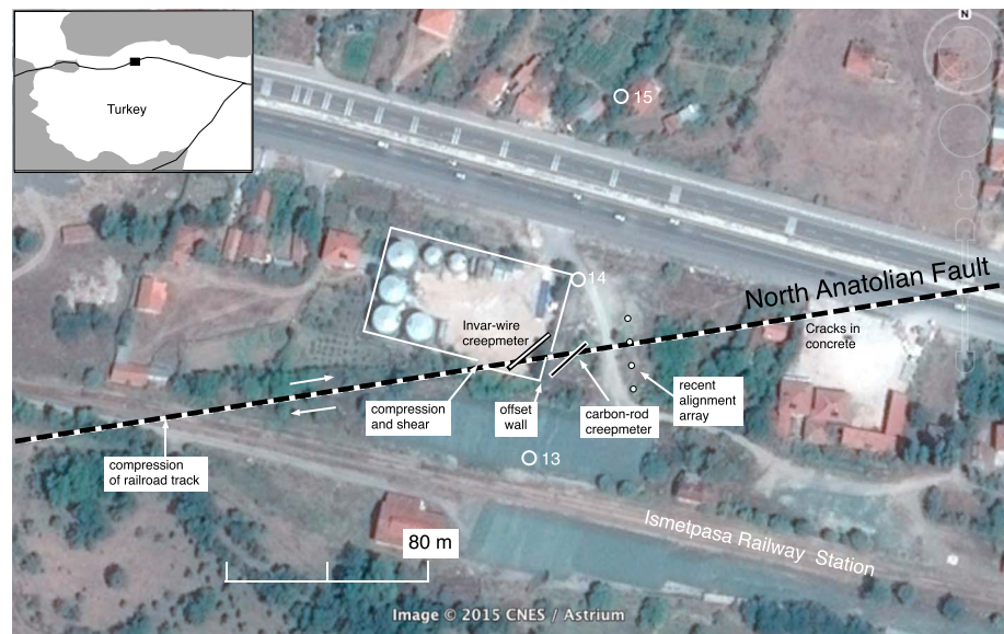
Figure 1. Google Earth view of the Ismetpasa maintenance yard showing the North Anatolian Fault and locations of invar and carbon fiber creep meters (40.870°N, 36.625°E). Nearby geodetic alignment array points 13–15 [Aytun, 1982] and the eastern wall of the maintenance yard cross the fault at 66°. The railroad crosses the fault at 24° in compression and has required occasional realignment and shortening to accommodate aseismic fault creep.
