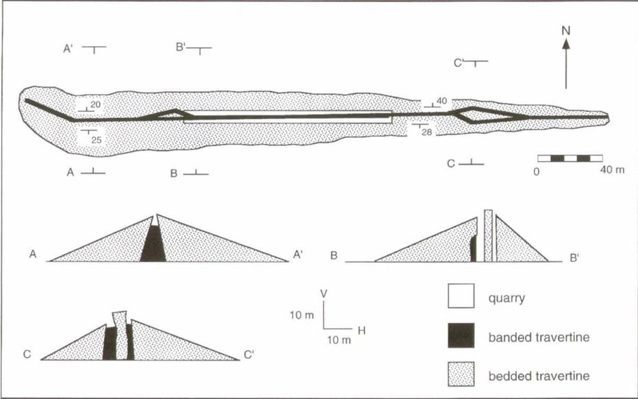
**Fig. 8.** Plan and profiles of the Çukurbag ridge (900 m east of Develi), the profiles emphasizing that Roman (and possibly later) quarrying has given rise to trench-like excavations where vertically banded fissure-ridge travertine has been selectively extracted.
