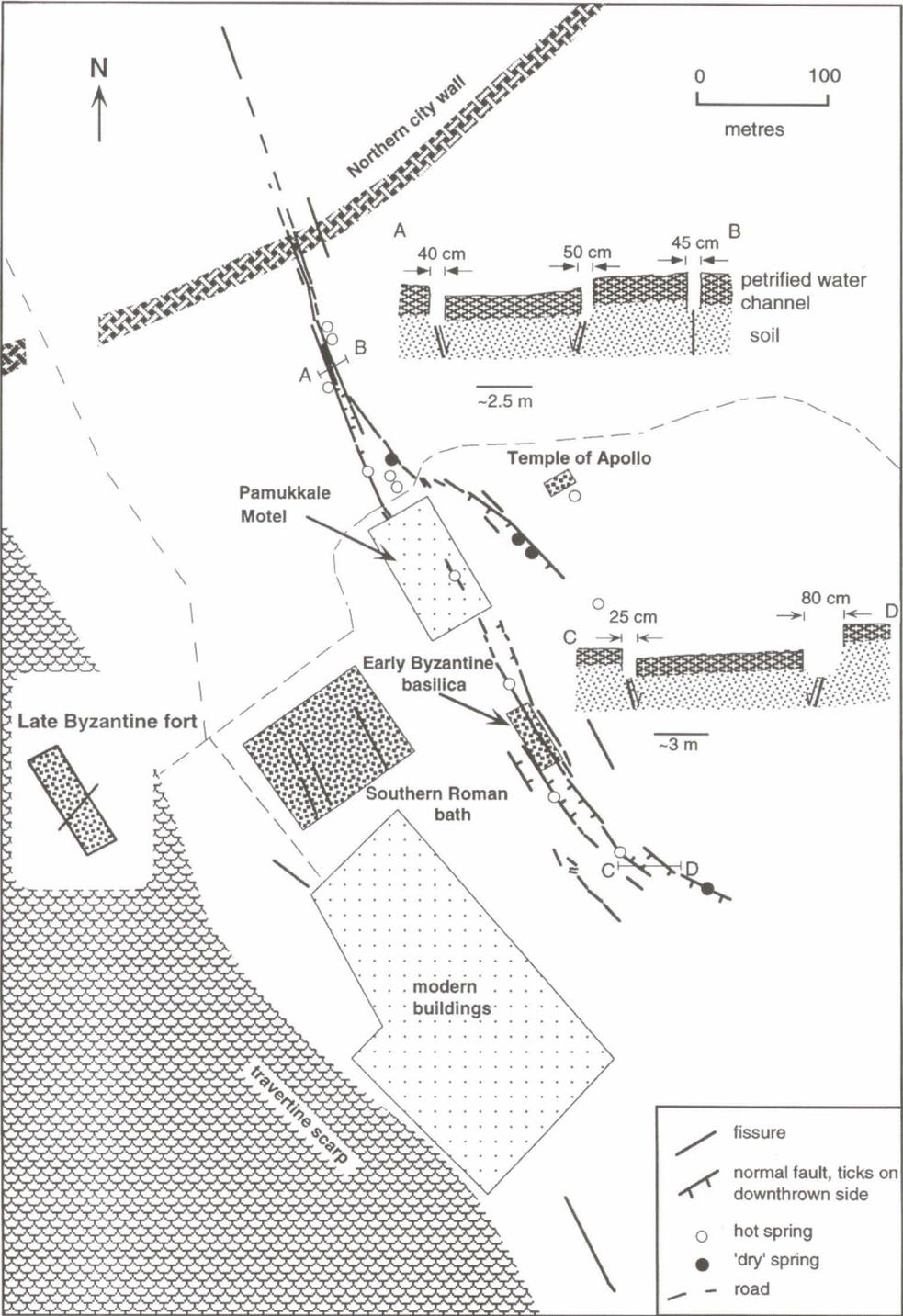
Fig. 13. Plan of the Hierapolis fault zone. The shapes of buildings are schematic and not all modern buildings are shown (after Hancock & Altunel 1997). It should be noted that in section A–B the petrified water channel is downfaulted in a mini-graben where it has been stretched over two normal faults that are oriented roughly at right angles to the line of the channel; the appearance of this mini-graben is illustrated in Fig. 15.
