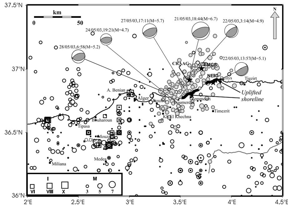
Fig. 3. Aftershock distribution (gray circles,  $M > 2$ ) from 21 May to 10 June 2003. Open squares show historical seismicity since 1365; open circles show instrumental seismicity since 1900. Stars are mainshock locations of the 21 May 2003 seismic event ( $M_w$  6.8) based on information from seismological centers. Focal mechanism solutions are CMT (Harvard) showing thrust faulting consistent with field observations and uplifted coastline.
