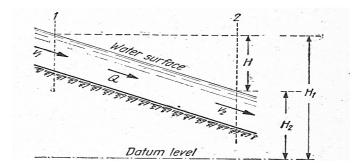
If the discharge at a velocity  $V_1$  through any section of a stream amounts to Q (m<sup>3</sup>/sec), the power of the flowing mass per second, with reference to any datum at a depth H<sub>1</sub> below the surface,
