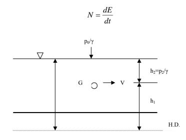
The total energy of any water particle of weight G, under pressure p, and moving at a velocity V, at an elevation  $h_1$  above a horizontal datum is, according to Bernoulli theorem,
