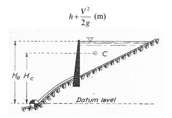
The total potential energy of the volume of water V stored in the reservoir is,
