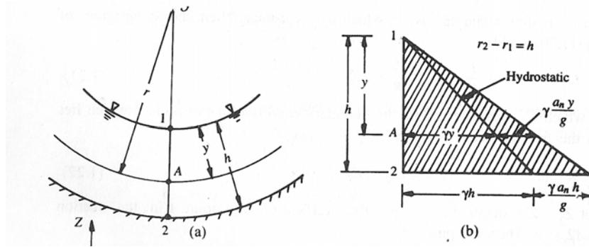
**Figure 4.8.** Concave curvilinear flow
