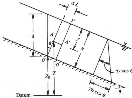
**Figure 4.7.** Pressure distribution in a channel with large slope
