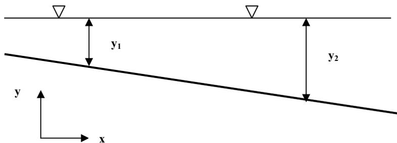
**Figure 4.2.** Non-Uniform steady Flow
