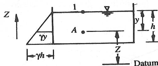
**Figure. 4.4.** Pressure distribution in still water
