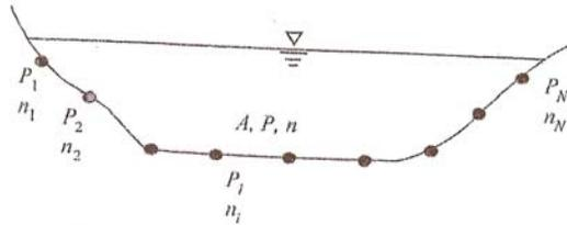
**Figure 4.5.** Multi-roughness type perimeter
