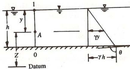
**Figure 4. 6.** Pressure distribution in a channel with small slope
