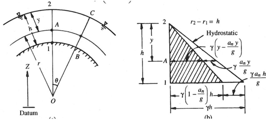
**Figure 4.8.** Convex curvilinear flow
