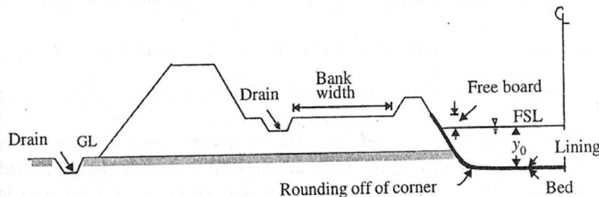
**Figure 4.10.** Typical cross-section of a lined canal
