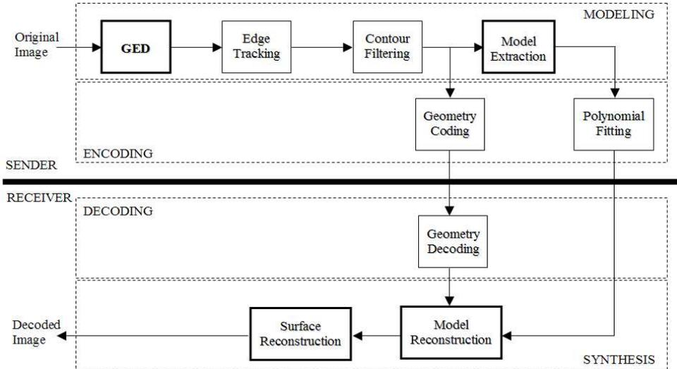
Figure 2. The generic architecture of the codec system.
