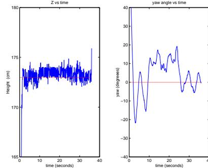
Fig. 9. The Results of the altitude and yaw Control Experiment with a Ground Camera based Direct Pose Estimation Method
