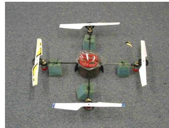
Fig. 1. A Four Rotor Model Helicopter, Quadrotor
