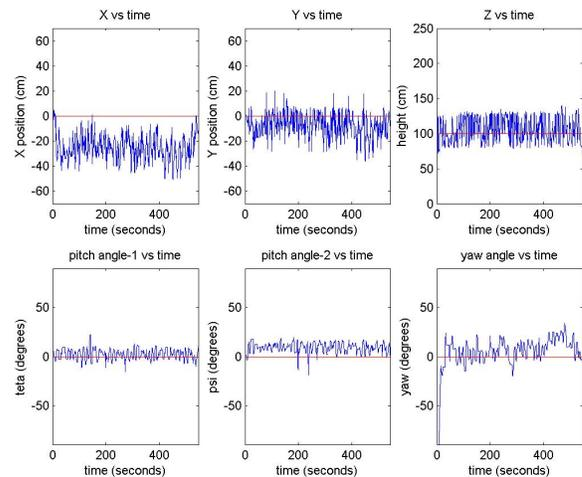
Fig. 10. The Results of the Height  $x$ ,  $y$  and yaw Control Experiment with Two-Camera Pose Estimation Method
