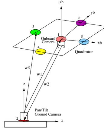
Fig. 3. Two-Camera Pose Estimation Method using a Pair of Ground and Onboard Cameras
