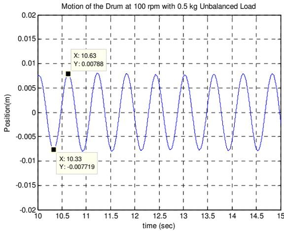
Fig.3. Motion of the drum on the y plane with 0.5 kg unbalanced load at 100 rpm.
