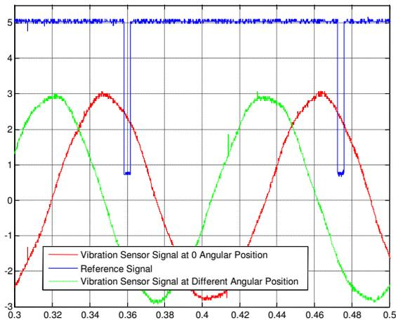
Fig. 10. Signals obtained during the experiment; the vibration sensor signal at zero (reference) position, the sensor signal obtained at a different angular position, and the reference signal.
