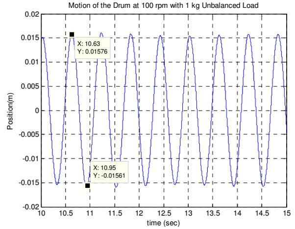
Fig.4. Motion of the drum on the y plane with 1 kg unbalanced load at 100 rpm.
