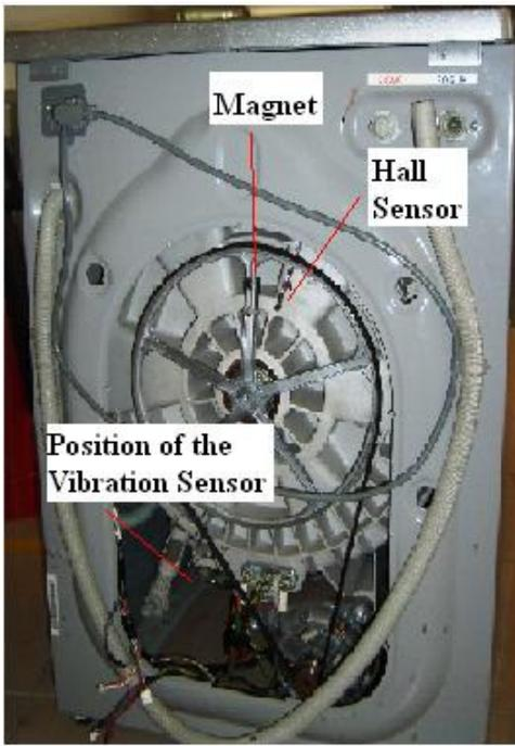
Fig. 9. The experimental setup showing the washing machine and the sensors.
