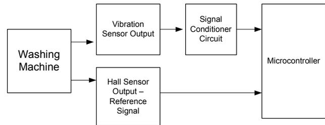
Fig. 7. Implementation of the unbalanced load measurement system.
