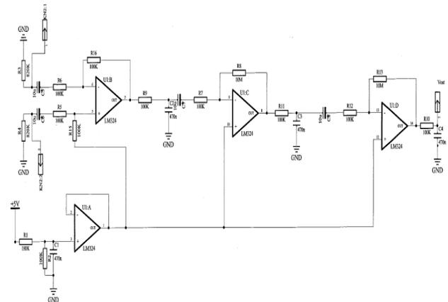
Fig. 8. Electronic circuit of the piezo electric sensor: The circuit amplifies, filters and conditions the signal.
