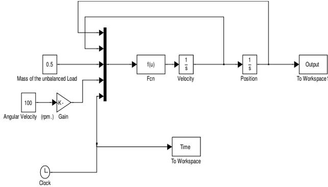
Fig. 2. MATLAB model of the unbalanced load and the measurement system.
