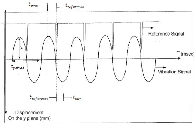
Fig. 6. The expected vibration signal at the nonzero angular position of the unbalanced load.
