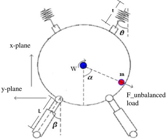
Fig. 1. Model of the unbalanced load in a horizontal load washing machine.
