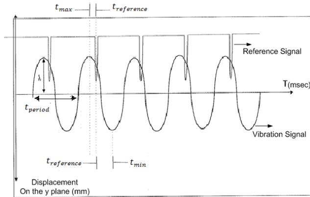
Fig. 5. The expected vibration signal at the zero angular position of the unbalanced load.
