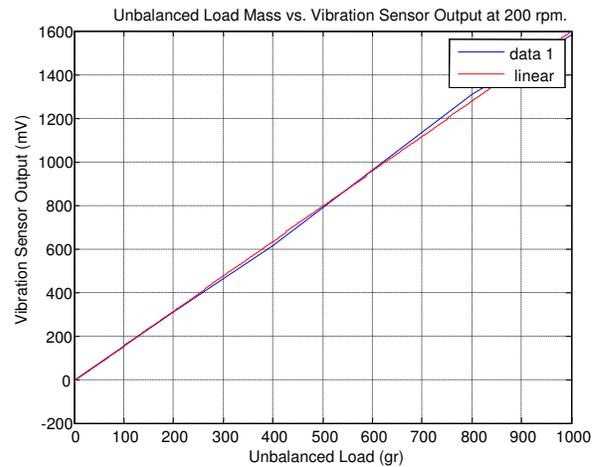
Fig. 11. Analyze of the calculated vibration sensor output with the different mass of the unbalanced load at 200 rpm.
