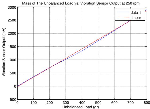
Fig.12. Analyze of the calculated vibration sensor output with the different mass of the unbalanced load at 250 rpm.
