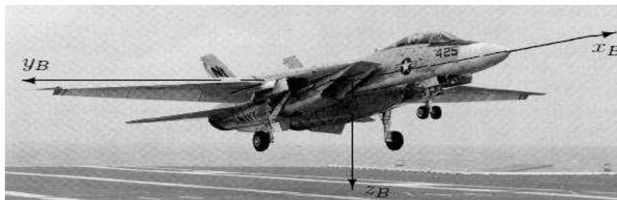
Figure 18. The Body Axes System [32]
