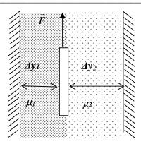
**Q.4.** A thin  $20\text{cm} \times 20\text{cm}$  flat plate is pulled at 2.4 m/s horizontally through a 6 mm thick oil layer sandwiched between two plates, one stationary and the other moving at a constant velocity of 0.8 m/s, as shown in the figure. The dynamic viscosity of oil is 0.027 kg/m·s. Assuming the velocity in each oil layer to vary linearly, determine the force that needs to be applied on the plate to maintain this motion. Here  $V_w$  refers to the velocity of the moving wall.
