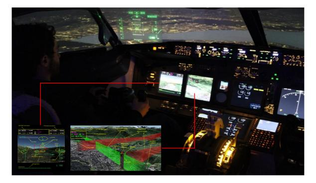
The developed automation support system is tested on a Boeing 737-800NG FNPT II level Flight Simulator with conceptual procedures enabling intent data exchange, automated flight control implementations, and synthetic vision based decision support system. The developed automation system offers persistent in-flight hazard and flight efficiency monitoring and tactical flight trajectory planning as a function of look-ahead time and dynamically changing environmental/operational conditions.
