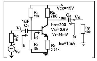
b) Vg is a sinusoidal signal the amplitude of which is 5mV and the frequency of which is the cut-off frequency at the high frequency region. Draw vg(t) and vo(t) for the same time-axis.
