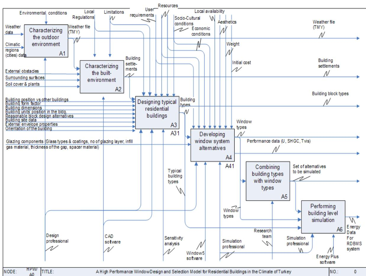
Figure 1: HiPerWin IDEF0 function model top-level diagram.
