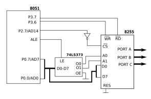
"All the ports of A, B and C are output ports" then the control word of the 8255 for the configurations ( $^{\circ}$  8255, page 3-100) is 10000000b=80h For P3.7 and P3.6 see  $^{\circ}$  80C51, page 6 and for 74LS373 (Latch) see  $^{\circ}$  74LS373. A program to send *FFh* to all ports:
