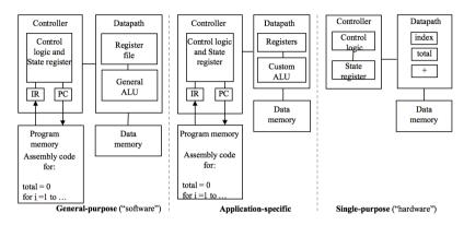
The architecture of the computation engine used to implement a system's desired
