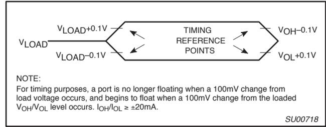
**Figure 20. Float Waveform**
