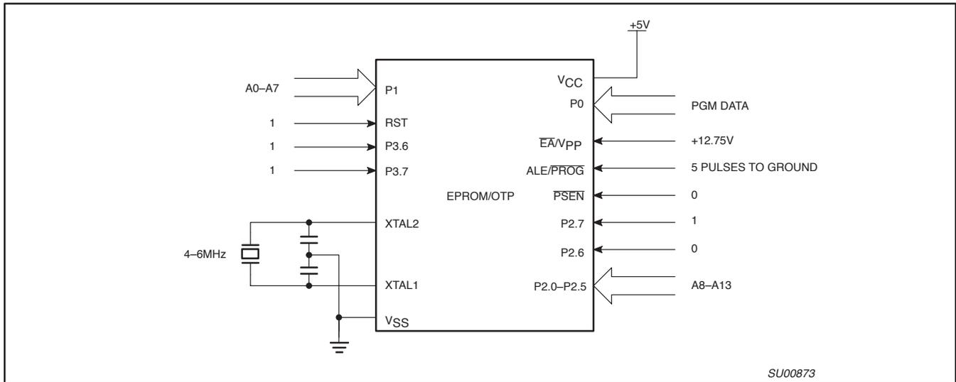
**Figure 26. Programming Configuration**
