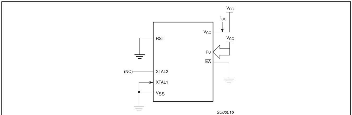
Figure 25.  $I_{CC}$  Test Condition, Power Down Mode
