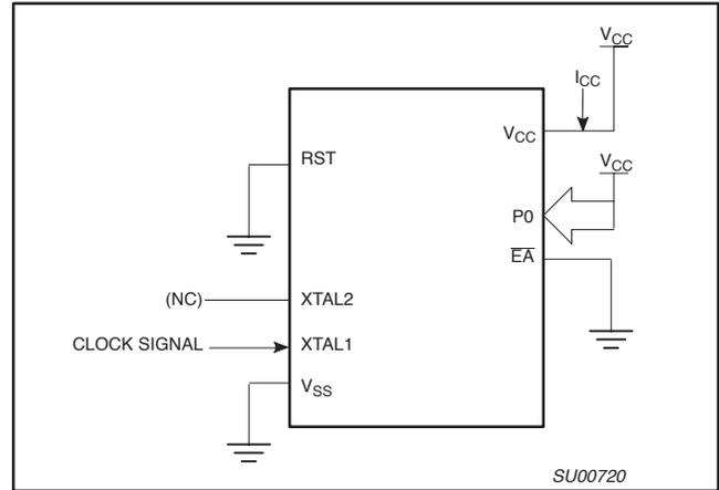
Figure 23.  $I_{CC}$  Test Condition, Idle Mode
