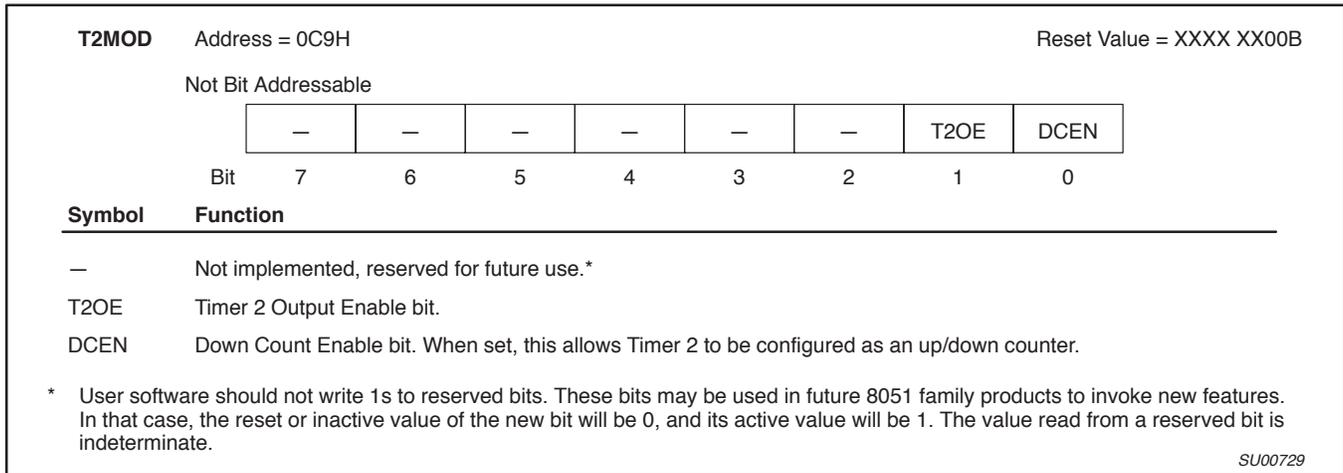
**Figure 3. Timer 2 Mode (T2MOD) Control Register**
