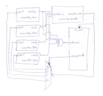
When interrupt is asserted, s1 register will give the counter number of interrupt in interrupt subroutine. When more than one interrupt is received, s1 register will give output of priority encoders. For priority\_encoder.v and conter.v please contact <a href="mailto:eabtioglu@gmail.com">eabtioglu@gmail.com</a>
