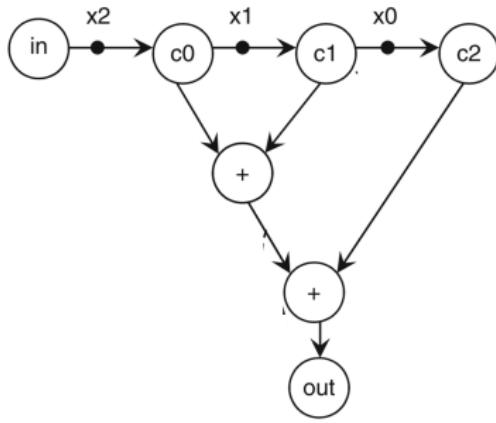
Not possible to introduce arbitrary initial tokens in a graph without following the rules for actor firing
