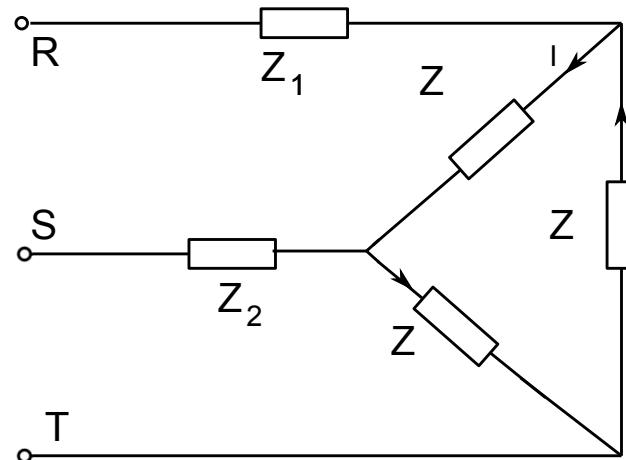
In a balanced 3-phase system,  $Z = 4 + j2$ ,  $Z_1 = \frac{2}{3}Z$  and  $Z_2 = \frac{1}{6}Z$  are given. For  $V_{RS} = V_{ST} = 20 + j10$ , calculate the currents  $I_R$ ,  $I_S$ ,  $I_T$ .
