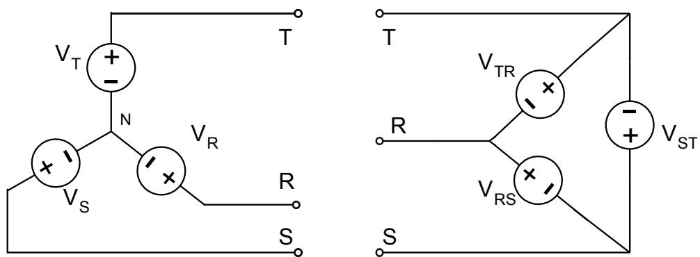
Phase Voltages of  $\text{Y}$ -connected source are the line-to-neutral voltages.
