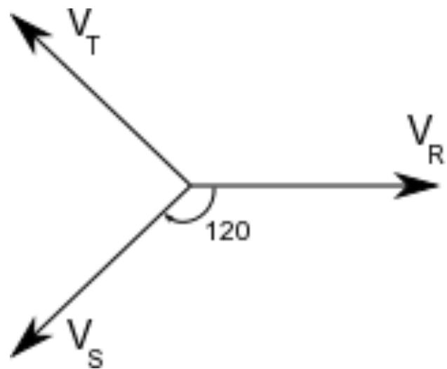
Phase Voltage of Y-connected source (The line-to-neutral voltages)
