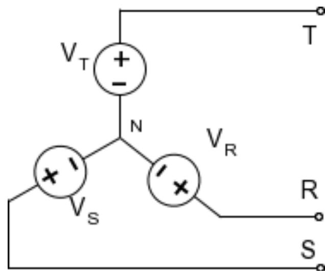
In  $Y$ -connection: line voltage and phase voltage are not identical !
