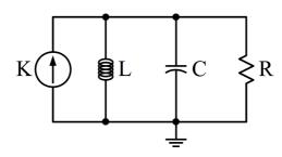
$$Y_{eq}(j\omega) = \frac{1}{j\omega L} + \frac{1}{R} + j\omega C = \frac{R + j\omega L - \omega^2 RLC}{j\omega RL}$$
