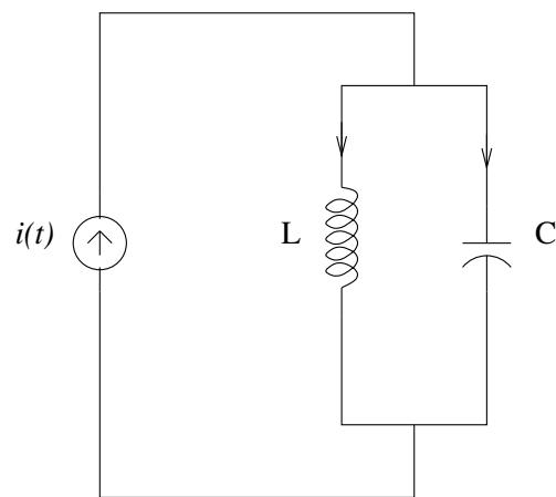
$$\begin{aligned} Li_L' &= V_C \\ CV_C' &= -i_L + i(t). \end{aligned}$$
