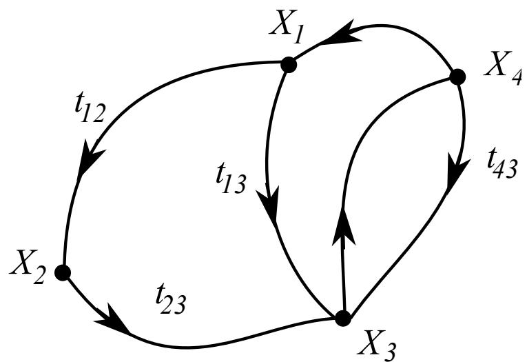
Signal-flow graphs are an alternative to block diagrams. They consist of edges which represent systems and nodes which represent signals. Multiple edges converging on a node implies summation.
