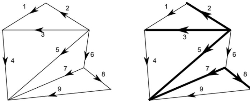
KCL equations based on Fundamental cut sets
