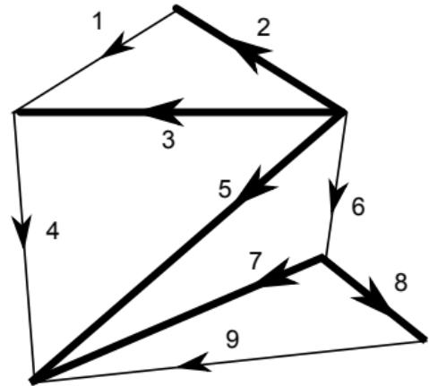
Fundamental cut sets of the tree  $G_T = \{2, 3, 5, 7, 8\}$  are  $G_{C2} = \{2, 1\}$ ,  $G_{C3} = \{3, 1, 4\}$ ,  $G_{C5} = \{5, 4, 6\}$ ,  $G_{C7} = \{7, 6, 9\}$ ,  $G_{C8} = \{8, 9\}$ .
