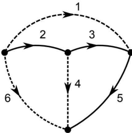
The links  $G_L = \{1, 4, 6\}$  for the chosen tree  $G_T = \{2, 3, 5\}$ . The Fundamental loop sets are  $G_{L1} = \{1, 2, 3\}$   $G_{L4} = \{4, 5, 3\}$   $G_{L6} = \{6, 2, 3, 5\}$ .
