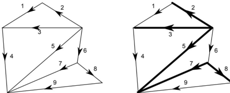
KVL equations based on the Fundamental loops
