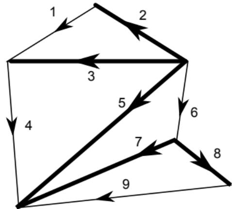
Fundamental Loop sets of the tree  $G_T = \{2, 3, 5, 7, 8\}$  are  $G_{L1} = \{1, 2, 3\}$ ,  $G_{L4} = \{4, 3, 4\}$ ,  $G_{L6} = \{6, 5, 6\}$ ,  $G_{L9} = \{9, 7, 8\}$ .
