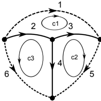
There are 3 meshes. Corresponding loop sets and mesh currents (loop currents)  $G_{M1} = \{1, 2, 3\}$  and  $i_{m1}$ :  $G_{M2} = \{3, 4, 5\}$  and  $i_{m2}$ ;  $G_{M3} = \{2, 4, 6\}$  and  $i_{m3}$ .
