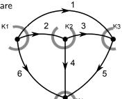
$G_{K1} = \{1, 2, 6\}, G_{K2} = \{2, 3, 4\}, G_{K3} = \{1, 3, 5\}, G_{K4} = \{4, 5, 6\}.$  If we apply KCL to the cut sets, we obtain
