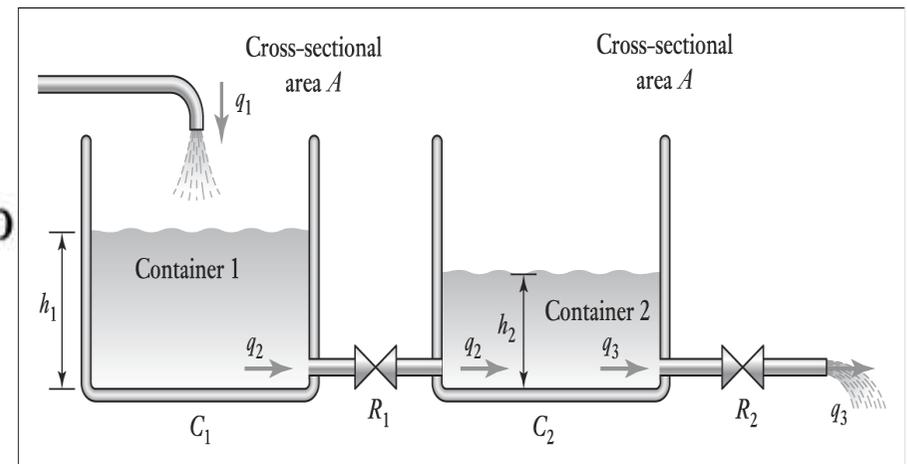
The rate at which liquid leaves the container  $q_3$  equals the rate at which it leaves the valve  $R_2$ . Thus for the resistor,
