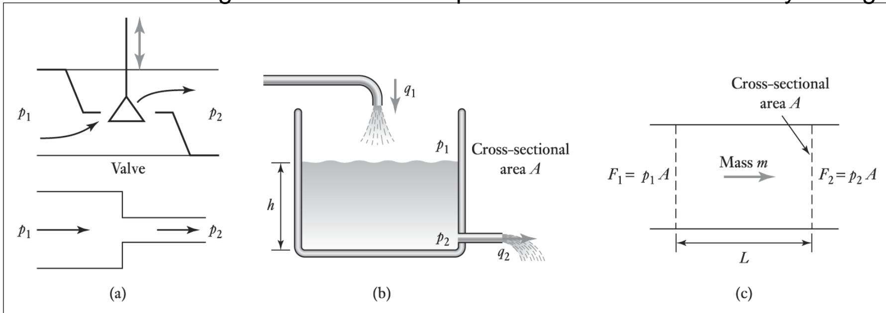
Figure 10.13 Hydraulic examples: (a) resistance, (b) capacitance, (c) inertance
